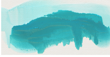
Figure 4: Paint runs down caused by tilting the device resulting in dripping. The dripping is not limited to be within stroke boundaries.
